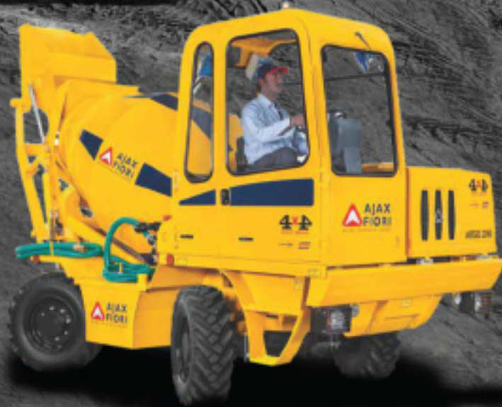
SELF LOADING MOBILE CONCRETE MIXER ARGO 2000 Capacity: 2 cbm
