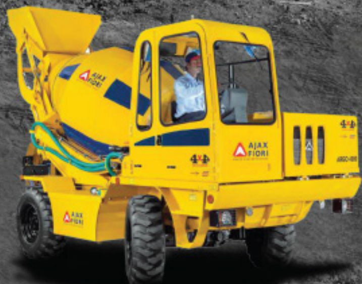
SELF LOADING MOBILE CONCRETE MIXER ARGO 4000 Capacity: 4 cbm
